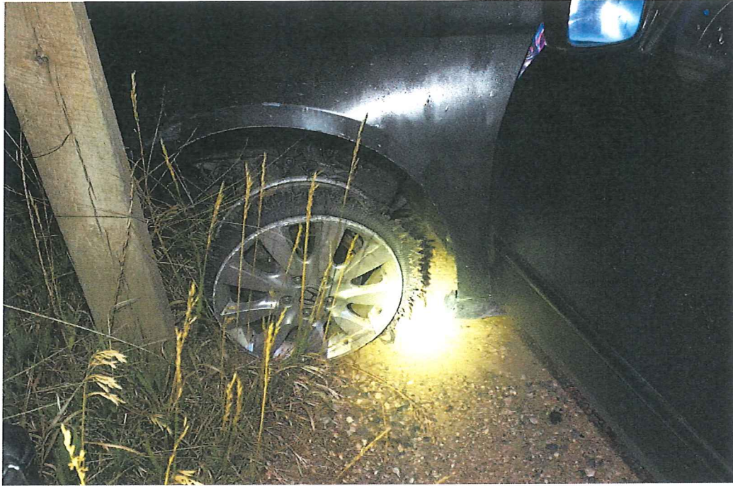
(Minugh's front left tire. Initial damage caused by tire deflation devices was exacerbated by continued driving at excessive speeds.)
