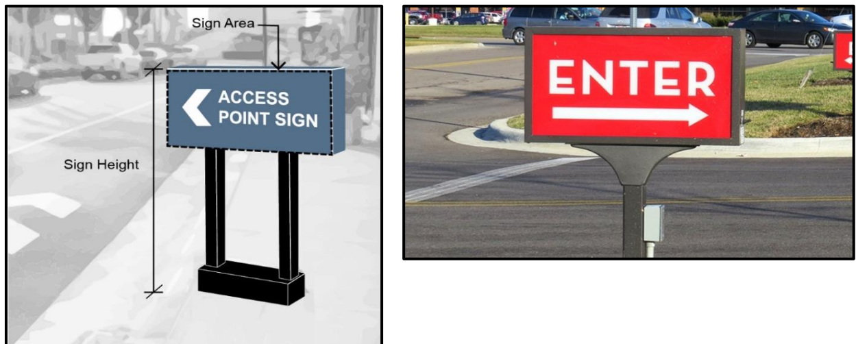
Figure 8-5: Access Point Signs
