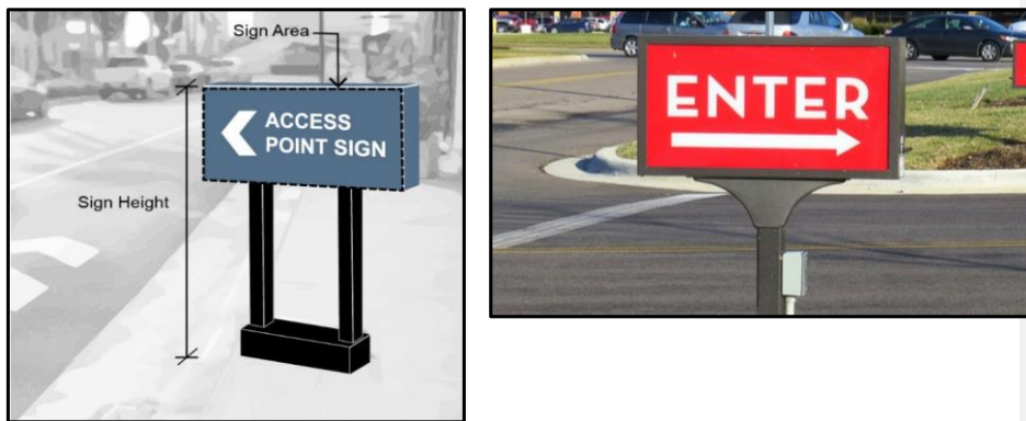
Figure 8-5: Access Point Signs
